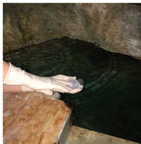
Figure 1. Water collection at the spring with aseptic procedure using sterile gloves and a sterile 50 ml syringe.
